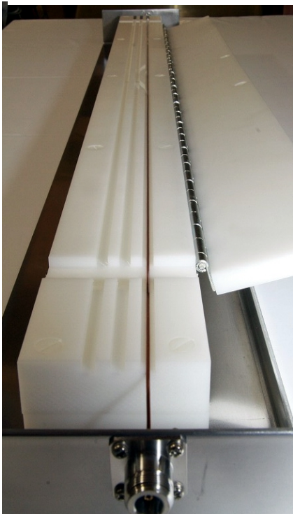
Figure H-4: RI 130/150 Test setup ( Configuration for a Twisted Wire Pair )
